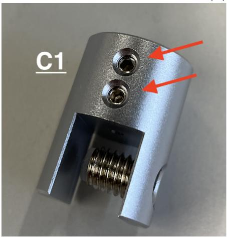
5. Insert a Solution hanging cable (C2) into the Solution screw block (C1). The end of the cable should align with the hole on the other side without sticking out.
